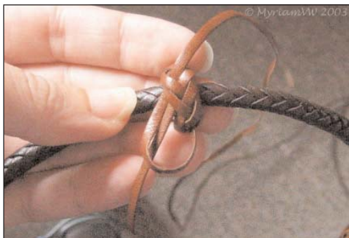
Fig. 13 - Over three (the third being the standing end), under two (make sure to lay the working end to the left of the standing end)
