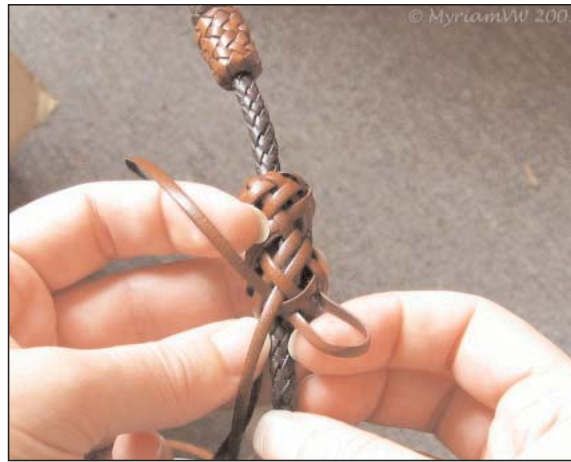
Fig. 32 - To start going back upward, take one thong and go over one and under two.
