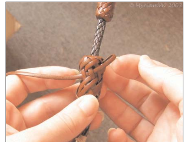
Fig. 30 - One more time with the fourth thong. Over two, under two (splitting parallels).
