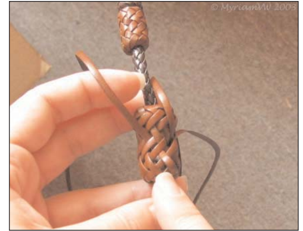
Fig. 39 - Once more with the fourth thong, over two, under two (splitting parallels). This completes the knot.
