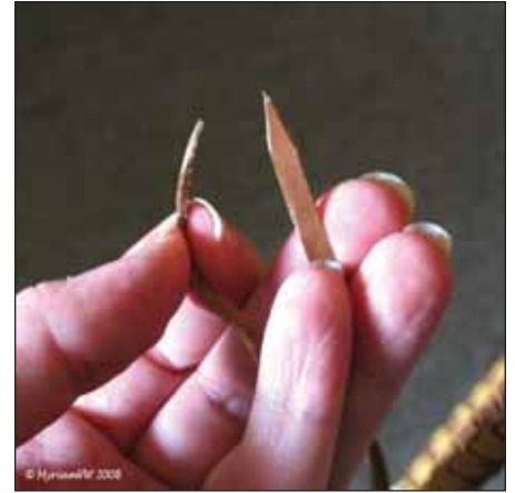
Fig. 12 - Now we need to prepare the ends of our strands for the lacing needles. First, skive the ends and cut them in an arrow shape.
