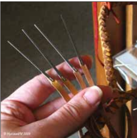
Fig. 13 - Then put a needle on each strand. Be sure to close the needles on the lace by tapping them with the mallet, else you'll be pulling the needles and the lace won't follow.
