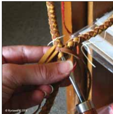
Fig. 14 - Now, for this part, you'll have to study the braid and see where each strand should go. Basically, you want to double over the previously braided part. Use the lacing fid to open up the space where you want to go. This makes it a little easier to pass the needle and lace through.
