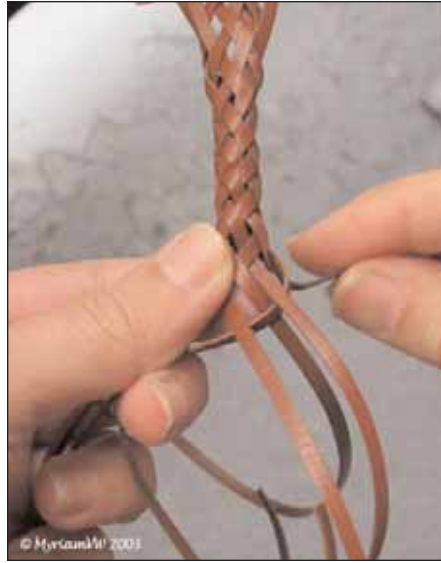
Fig. 8 - Weave the thong in, pull snug, hold all thongs except the first one you weave over and pull tight and even.
