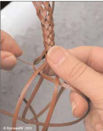
Fig. 4 - Grab the working end with free fingers from the other hand and bring through the path you just opened.
